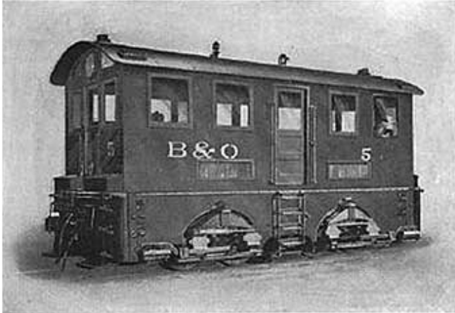
Hall of 100-ton Electric Locomotive built by General Electric Company for B. & O. Ry. Co. The complete locomotive may be operated from either end by means of one controller.
