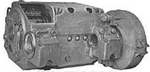
G. E. 69 Motor, 200 H.P. With Cover Removed
